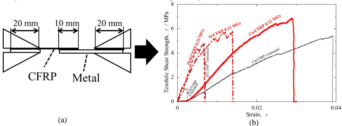
Fig. 1 Schematic drawing of shearing test (a) and tensile shear stress – strain curves at low accumulative probability of the shear strength ( $P_s=0.15$ ) of CFRP/Metals (Cu, Al and 18-8) laminated sheets with and without 0.22 MGy-HLEBI (b).
